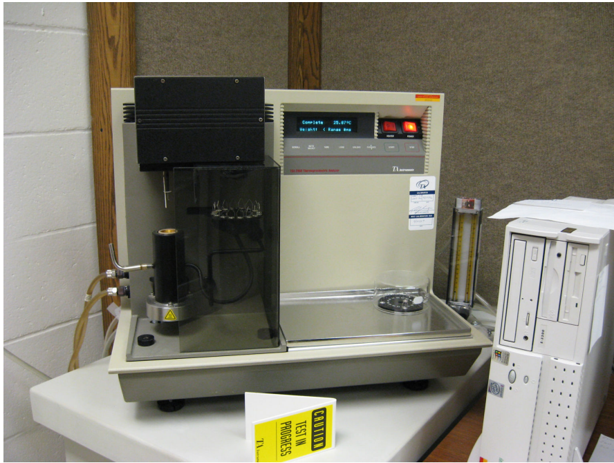
Thermo-gravimetric analyzer (TA Instruments - TGA 2950)
