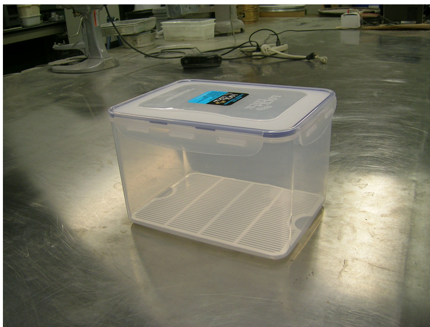
Airtight container for the storage of mortar-bars in 1N NaOH solution at 80°C
