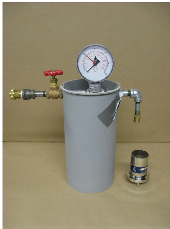
Water pressure regulator and ASTM No. 325 sieve for 45 µm residue analysis
