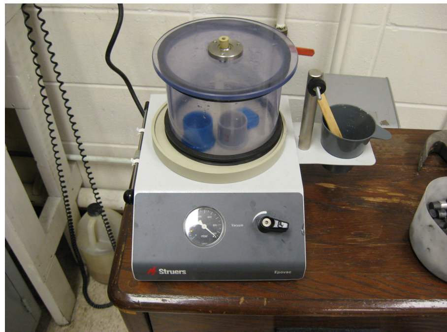
Unit for epoxy impregnation under vacuum
