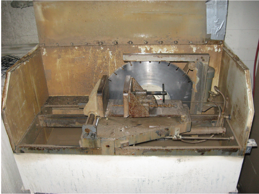
Concrete saw to cut 100 \times 50 mm ( 4 \times 2 in.) sections for rapid chloride permeability
