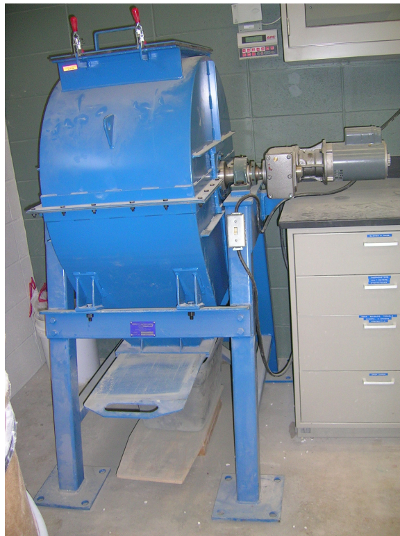
Laboratory type ball mill with dust control casing
