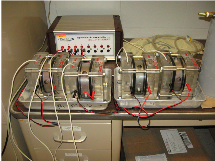
Permeability cells and data acquisition unit for rapid chloride permeability testing
