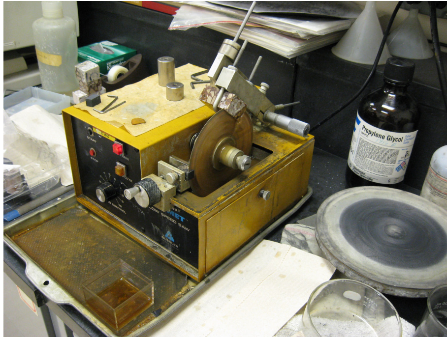
Slow speed saw for detailed sectioning of concrete for microstructural investigation
